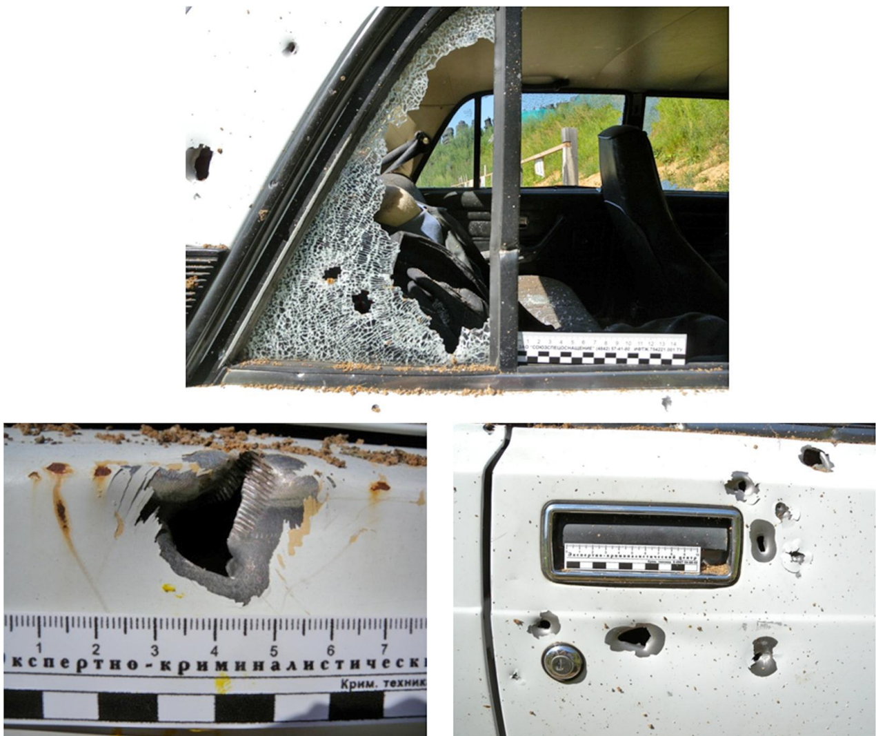
Fig. 49. Scale images of explosive submunitions traces on the right side of the vehicle
