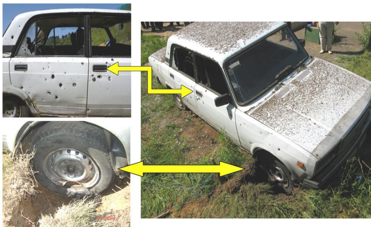
Fig. 48. Localization of lesions on the right side of the vehicle (arrows indicate the enlarged photographs of similar parts of the vehicle)
